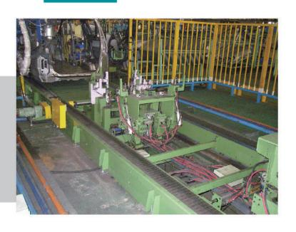
升降倒料作業系統(鋁壓鑄、螺絲業適用) Automated delivery system for Die Casting and screw manufacturing industry
